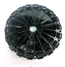
Step 6: Insert a M3 nylock nut and screw it in with its M3 x 10mm SHCS until all holes have been filled.
