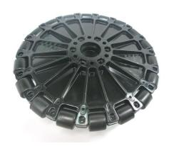
Step 5: One at a time place a M3 nylock nut into 4 of the holes in a "plus-shaped" form on the omni web that is underneath. On the omni web that is above insert 4 M3 x 10mm SHCS so they align with the ones underneath. Screw them in loosely as you do so, but tighten them all once all four screws are inserted.
